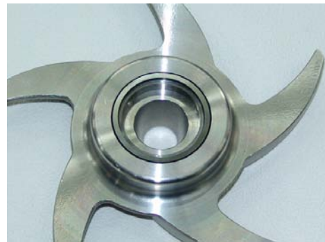
Pin for seal shall be complied to notch of seal ring.
