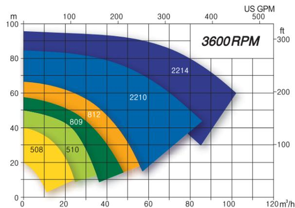
Performance data refer to water at 20°C, Permissible tolerance ±5%
